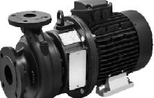
Materials and building features Pump body / Mechanical seal housing / Motor bracket: Cast-iron GG20 with anti-corros ve coating Suction/delivery ports: according to standard EN1092-2 Impeller: Cast-iron GG20 with cataphoresis coating Pump shaft: Stainless steel AISI 304 Mechanical seal: Carbon / Ceramic / NBR
